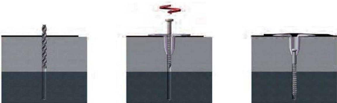
1. Drill a hole of required diameter and depth.
